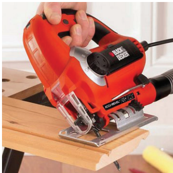
38-rasm. Elektr lobzik kesish burchagining og'ishi
